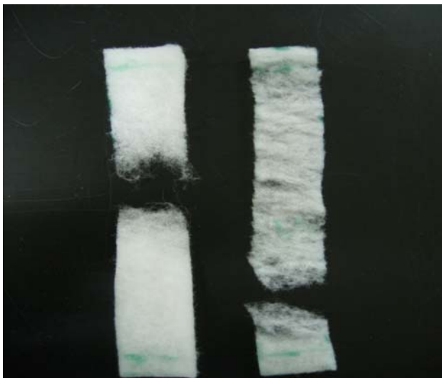
Fig. 9 Broken images of nonwovens after tensile loading (a) air folding and (b) mechanical folding types
